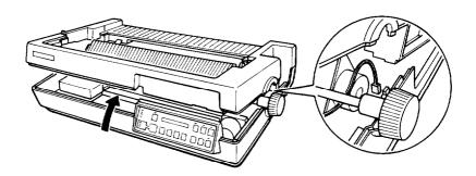
5. Remove the connector labelled **CN21** as shown in the following illustration. Then remove the upper case completely.
